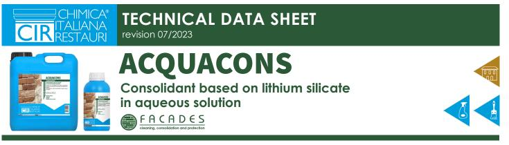
**DESTINATION** > Natural stones of any kind and absorbent building products. Particularly suitable for consolidating cement and concrete substrates.
